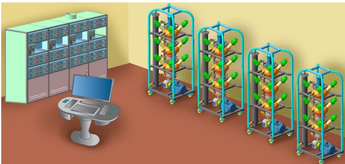
Fig. 2. Appearance of the facilities for cavitation hydrogenation of hydrocarbon feedstocks "Potok-7MI-200". They are based on toroidal-type reactors and 48 emitters of a pezostriktype. The facilities are equipped with a system of monitoring and control over the pumps and sensors.
