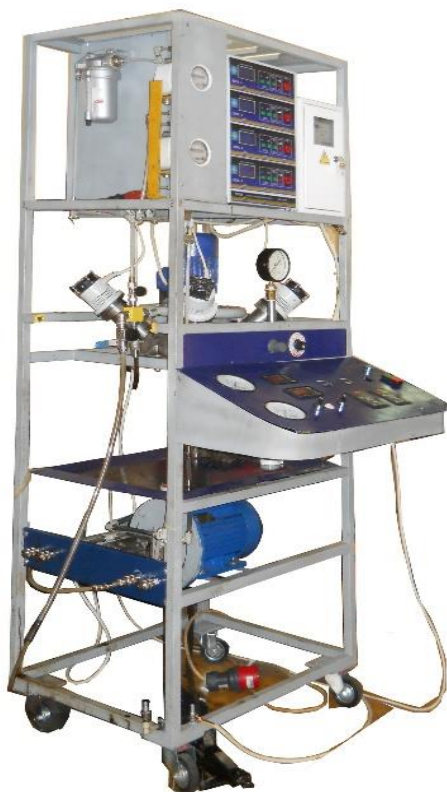
Fig. 1. Appearance of the laboratory installation "Potok-7M", which was used for the restructuring of Zhangurshi oil.
